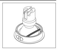
Put the lamp between springs as shown in the image.
