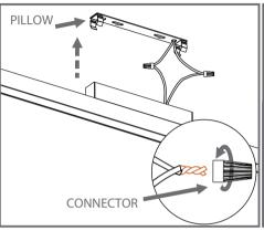
2º Use the connectors inside to finish the electrical installation.
